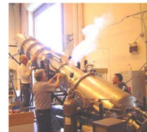
Snail pump under test at LANL.
